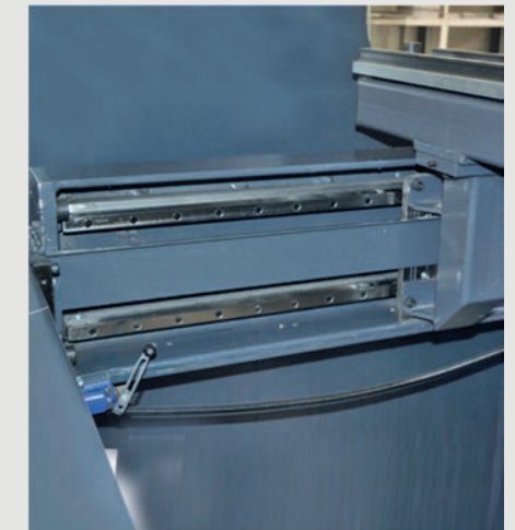
Linear Guided Stronger Back Gauge X Movement
