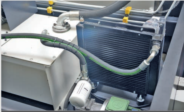
Hydraulic Oil Cooling System
